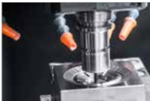
Spindle Nozzle & Cutting Air Blow
