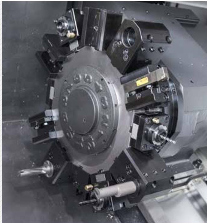
BMT turret applied in L300M series, with 4 screws solidly fastening the holder, shows outstanding performance in milling, drilling and tapping during heavy duty cutting.
