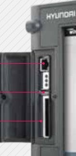
Easy input/output of programs is possible with the use of USB memory card, CF memory card and LAN.
