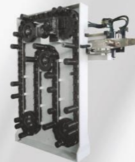
RV TOOL MAGAZINE : STANDARD 60 TOOLS. OPTION 90 TOOLS AND 120 TOOLS
