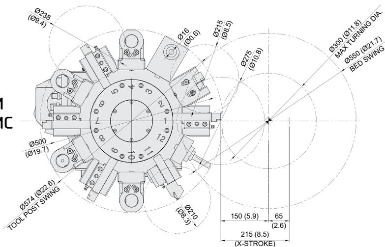
If the tool is placed differently from the picture above, it may interfere with the chuck when applying the O.D Extension holder.
