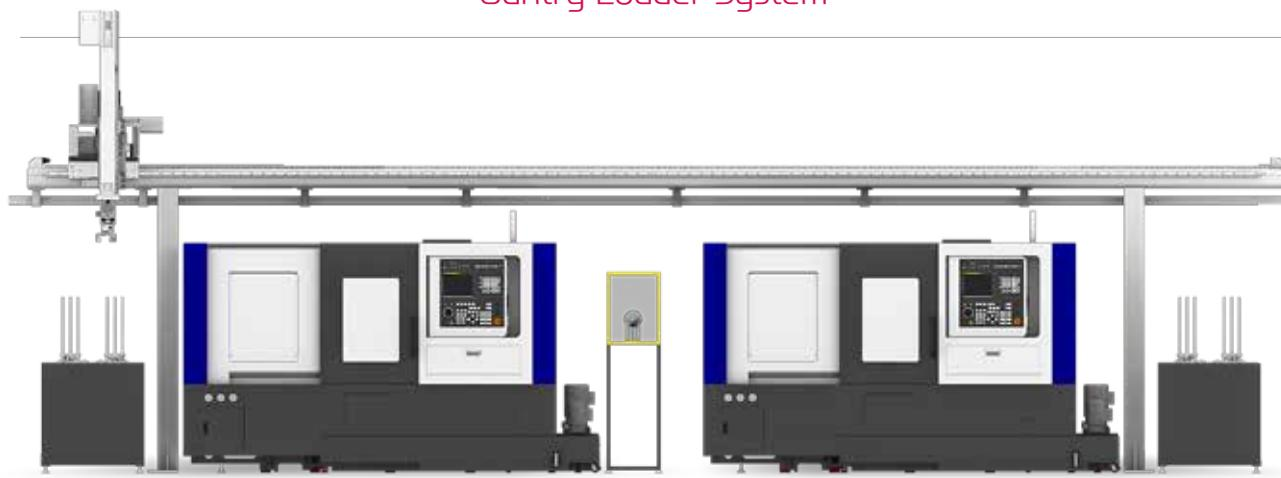
**Gantry Loader Machining Process**
